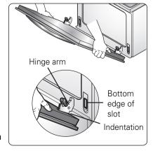
arm must be fully seated into the bottom of the slot.
